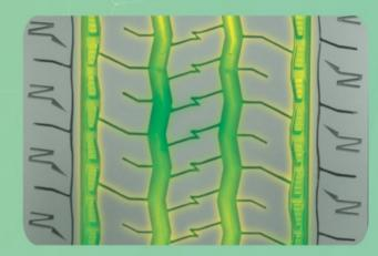
Shoulder Stiffness Hold Technology (SSHT) - Less uneven wear
